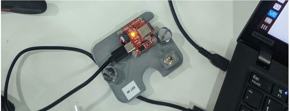
Figure 12: The electronics board plugged into a power source via the charging wire. The 'orange LED' shows that the charging has started.
